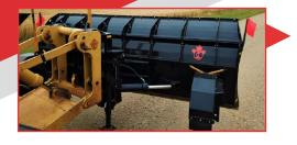
Has 2 adjustable legs to assist with disconnect Has wheel or button shoes for winter use Angle 30 degrees left or right 1 ½" or 2" Quick Attach pin Install bolt on top for snow application Weight – 2987 lb
