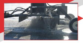
Mills washboards, ice, and removes rock from road surface
