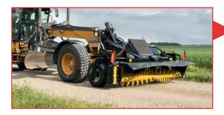
The Capital I Pull Type Sod Mulcher performs the same work as the Grader Mount Sod Mulcher
