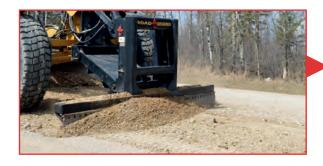
The Road Groomer attachment cuts washboards, ice, and removes rocks from road surface
