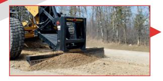
Cuts washboards, ice and removes rock from road top
