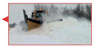
Hydraulically controlled bottom edge folds ahead and back.
