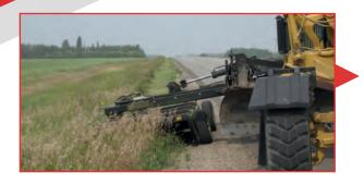
Controlled entirely from cab using hydraulics
