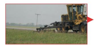
Loose link mounting assembly allows mower to float over obstacles
